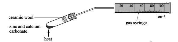
A mixture containing 0.27 g of powdered zinc and 0.38 g of powdered  $CaCO_3$  was heated strongly for two minutes. The volume of gas collected in the  $100 \text{ cm}^3$  syringe was then measured. The experiment was then repeated.
